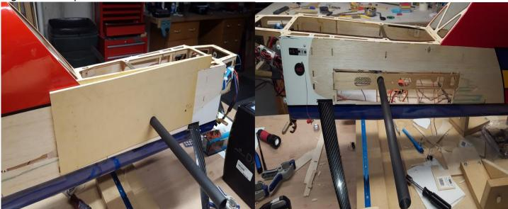
The transfer template was then used to rough in new interior structure to the left-side fuselage with the wing tube sleeve in approximately the correct location. Plywood rings were fabricated with close tolerance holes to the wing tube sleeve outer diameter, and the left structure hole opened slightly to allow
