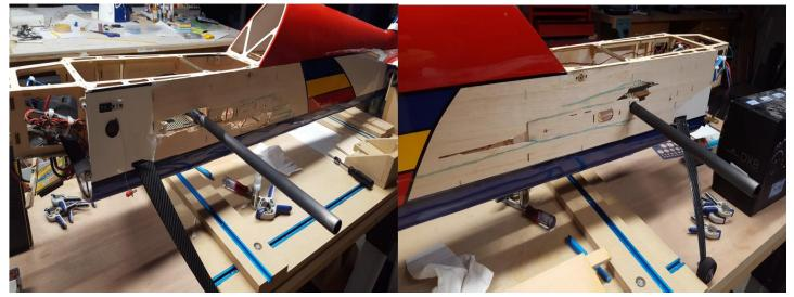
transfer template from ½" MDF panel with a close tolerance hole to match the wing tube. Basswood strips were glued to register the panel relative to the canopy sill, as shown in the photo below. Matching basswood strips were then glued on the opposite surface (near side in photo), even with the initial canopy sill registration strips.
