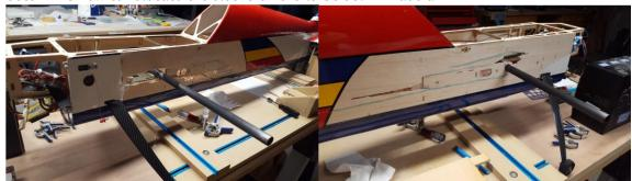
transfer template from ¼" MDF panel with a close tolerance hole to match the wing tube. Basswood strips were glued to register the panel relative to the canopy sill, as shown in the photo below. Matching basswood strips were then glued on the opposite surface (near side in photo), even with the initial canopy sill registration strips.
