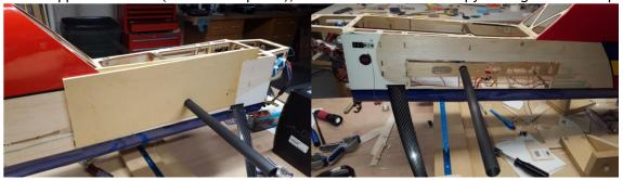
The transfer template was then used to rough in new interior structure to the left-side fuselage with the wing tube sleeve in approximately the correct location. Plywood rings were fabricated with close tolerance holes to the wing tube sleeve outer diameter, and the left structure hole opened slightly to allow refinement of that side of the sleeve. Other damaged internal structure was either repaired or replaced as needed.
