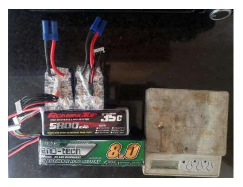
Although the thought of carrying around 12 cells in a model designed for 6 sounds heavy but Li-Ion packs configured in a 6S/2P 8000mAh weighed in at 2 pound. My Turnigy 6S 8000mAh 25C Lipo weighs in at 2 pounds 8 onuces and the RoaringTop 6S 5800 35C weighs in a 1 pound 11 ounces. Flight testing will start soon.
