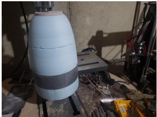
With the initial hand sanding done time to temporarily glue ends on to mount it to the drill press for more sanding. The center, for ducting will have to be removed. I haven't decided if I will cut it in half or drill a starter hole for the hotwire.
