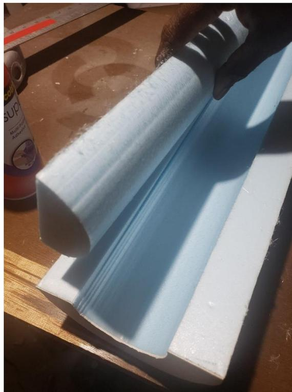
Section 2 (cylinder) cut and rolled over the intake duct cut and removed. The process is fairly quick but it will slow when I get to the final sanding and finishing.
