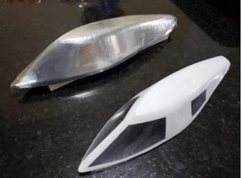
Note, that the heated deformed plug shows the inner surface of the 3D printing process.
